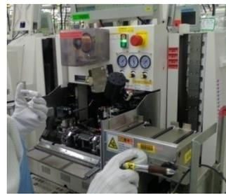
WB工序劈刀加载
